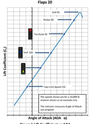
Figure 1 Lift Coefficient vs AOA
