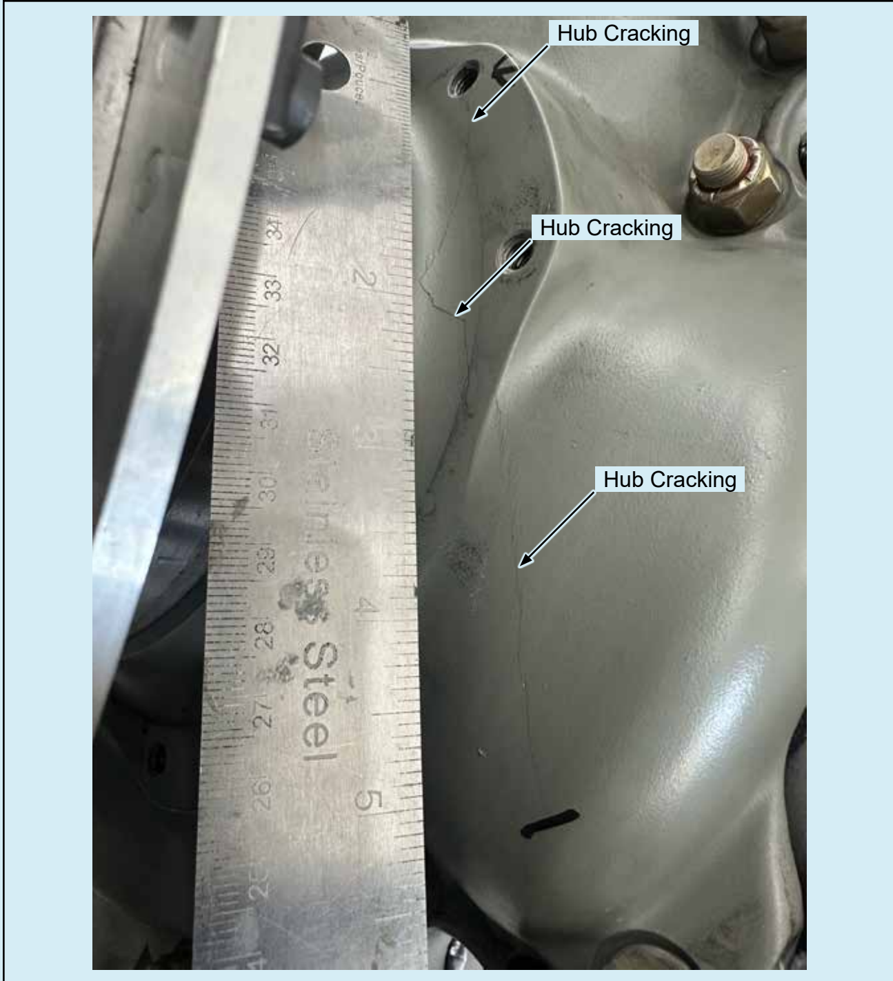
Hub Cracks Figure 1, page 1 of 2
